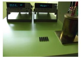
Figure 4. The measurement of the electrical resistance by four-point method.
