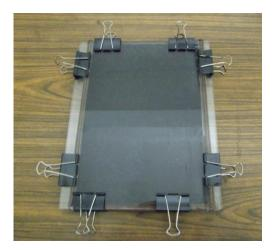
Figure 1. The formed fabric reinforced epoxy composite by wet lay-up method.
