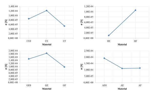
Figure 6. The electrical conductivity of the composite materials measured by four-point method.
