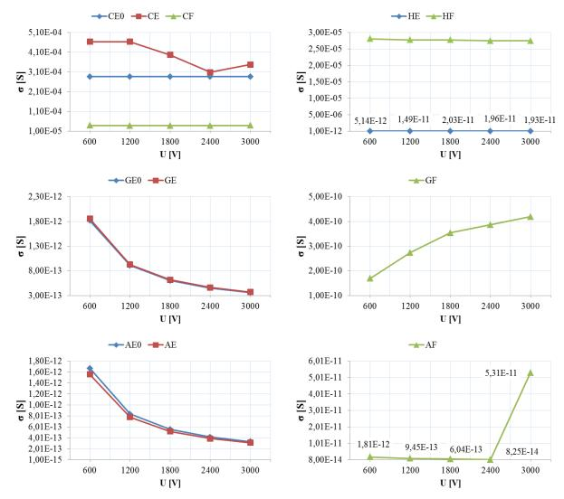
Figure 5. The electrical conductivity of the composite materials measured by two-point method.
