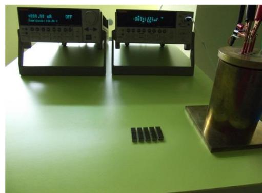
**Figure 4. The measurement of the electrical resistance by four-point method.**
