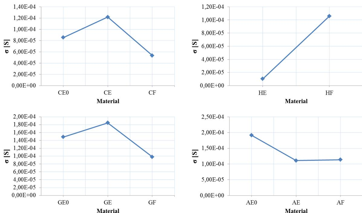
**Figure 6. The electrical conductivity of the composite materials measured by four-point method.**
