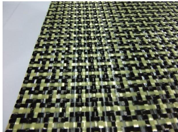
**Figure 2. The special hybrid fabric made of three alternating fibers (carbon, aramid and glass) and tinned copper wire.**
