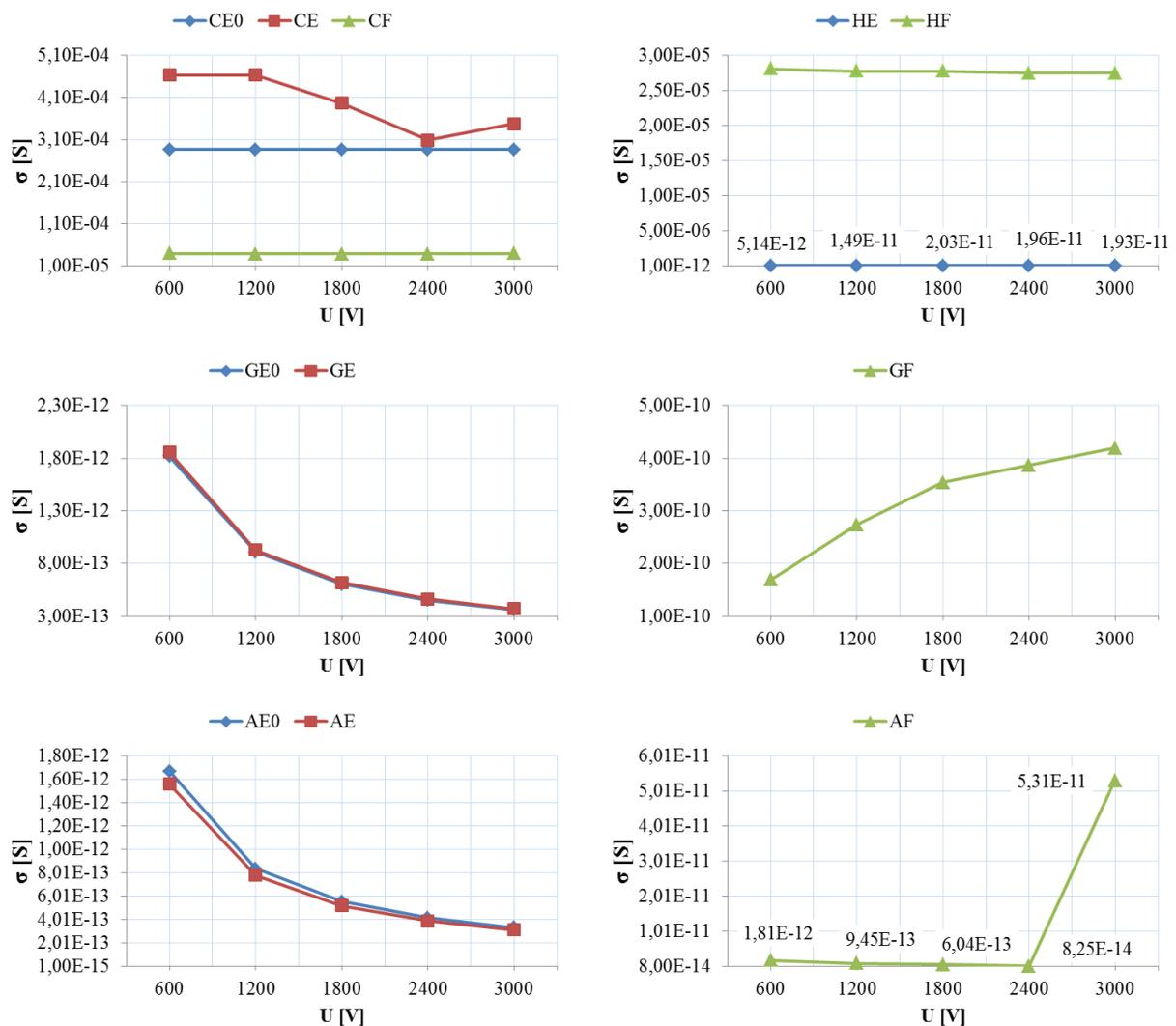
**Figure 5. The electrical conductivity of the composite materials measured by two-point method.**
