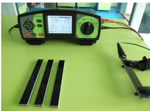
**Figure 3. The measurement of the electrical resistance by two-point method.**
